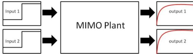
Fig. 4 Open-loop step test of MIMO plant
