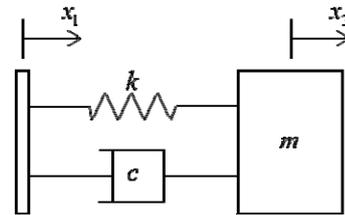
Fig. 3 An m-c-k system as an illustrative example.
