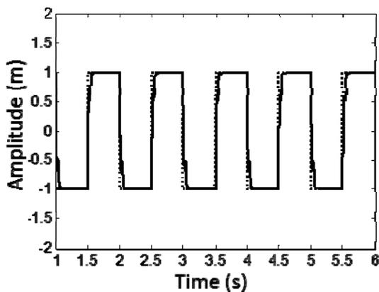
Fig. 8 Nominal plant with the input shaper: (dash) reference  $r$ , (solid) output  $y$ .
