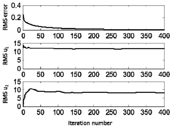
Fig. 11 (Top) Root-mean-square (RMS) value of the error  $e = y_m - y$ . (Middle) RMS value of the feedback control effort  $u_1$ . (Bottom) RMS value of the ILC control effort  $u_2$ .
