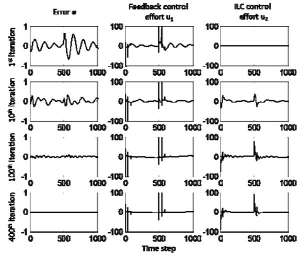
Fig. 12 The error  $e$ , the feedback control effort  $u_1$ , and the ILC control effort  $u_2$  during the 1<sup>st</sup>, 10<sup>th</sup>, 100<sup>th</sup>, and 400<sup>th</sup> iterations.
