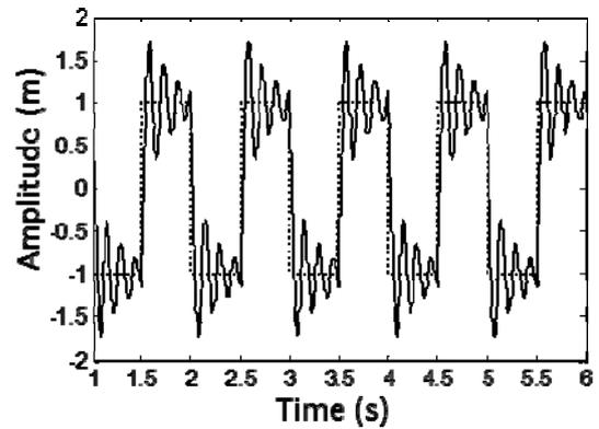
Fig. 9 Perturbed plant with the input shaper: (dash) reference  $r$ , (solid) output  $y$ .
