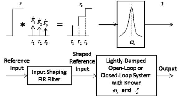
Fig. 1 Implementation of input shaping technique.
