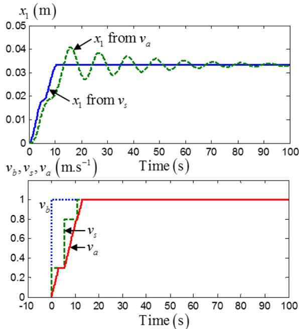
Fig. 6 (Top) Unit-step velocity response of the two-mass rigid-flexible system. Solid line is shaped response. Dash line is response under acceleration limit. (Bottom) Unit-step baseline velocity command  $v_b$ . Shaped command  $v_s$ . Acceleration-limited command  $v_a$ .
