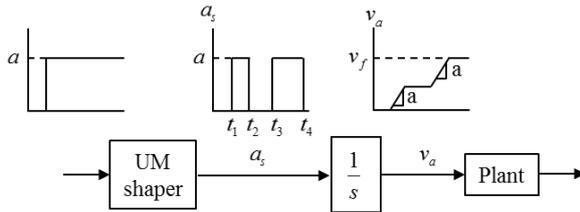
Fig. 1 UM shaper design to avoid violating acceleration limit.
