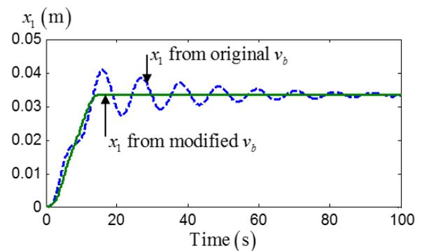
Fig. 9 Unit-step velocity response of the two-mass rigid-flexible system. Solid line is the result from
