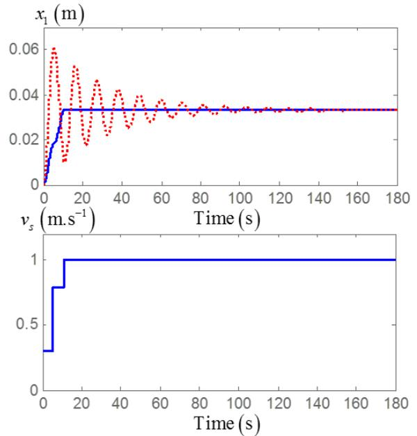
Fig. 4 (Top) Unit-step velocity response of the two-mass rigid-flexible system. Solid line is shaped response. Dash line is unshaped response. (Bottom) Shaped unit-step velocity command.
