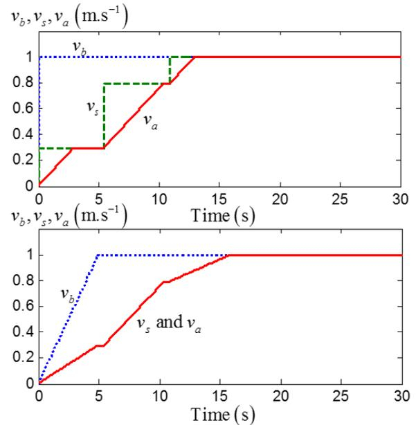
Fig. 8 Unit-step baseline velocity command  $v_b$ . Shaped command  $v_s$ . Acceleration-limited command  $v_a$ . (Top) Original baseline command. (Bottom) Modified baseline command.
