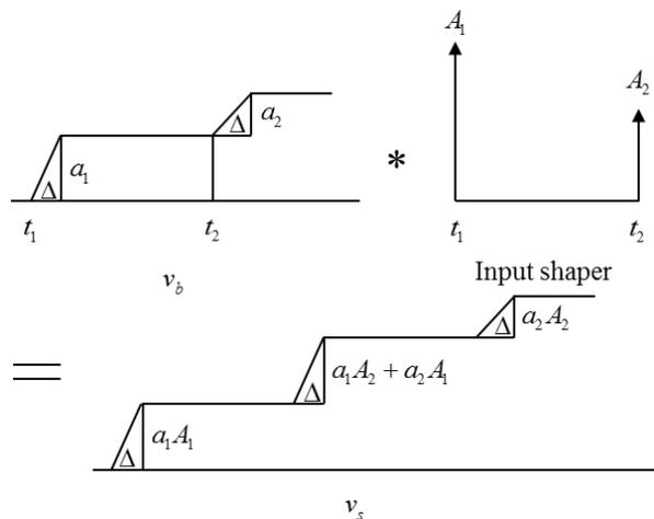
Fig. 10 Convolution between modified baseline command with two steps and input shaper's impulse sequence.
