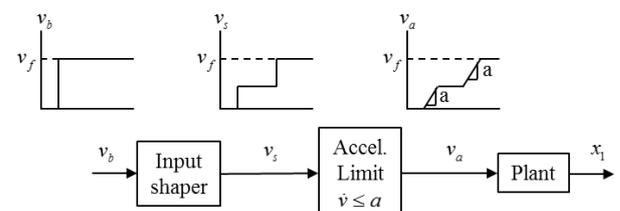
Fig. 5 Input shaping under acceleration limit.
