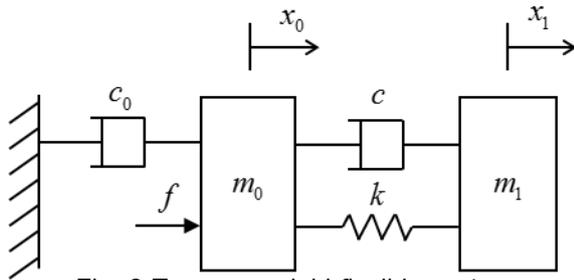
Fig. 2 Two-mass rigid-flexible system.
