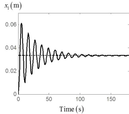
Fig. 3 Unit-step velocity response of the two-mass rigid-flexible system.
