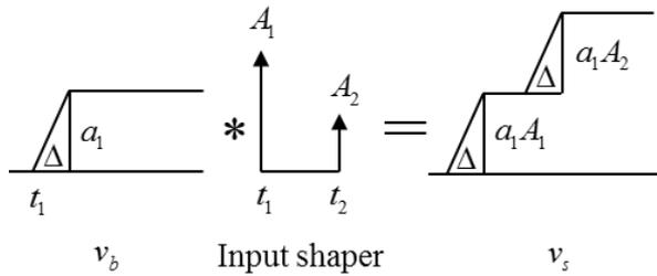
Fig. 7 Convolution between modified baseline command and input shaper's impulse sequence.
