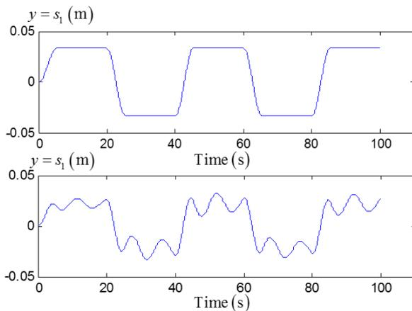
Fig. 7 (Top) Plant output when the plant model is perfect. (Bottom) Plant output when the model is uncertain.
