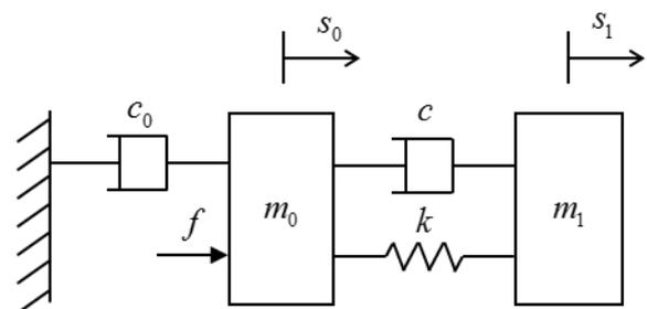
Fig. 1 Two-mass rigid-flexible system.
