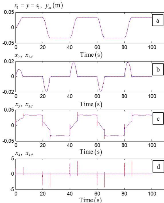
Fig. 8 States and their desired values. (a) System output  $x_1 = y = s_1$  and its desired value  $y_m$ . (b) State  $x_2$  and its desired virtual control  $x_{2d}$ . (c) State  $x_3$  and its desired virtual control  $x_{3d}$ . (d) State  $x_4$  and its desired virtual control  $x_{4d}$ .
