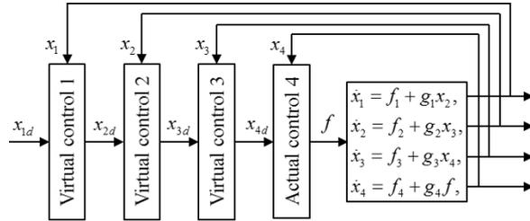
Fig. 3 State-feedback backstepping control.
