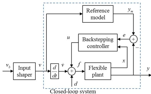
Fig. 4 Proposed model reference input shaping using state-feedback backstepping control.
