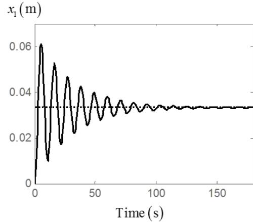
Fig. 2 Impulse response of the two-mass rigid-flexible system.
