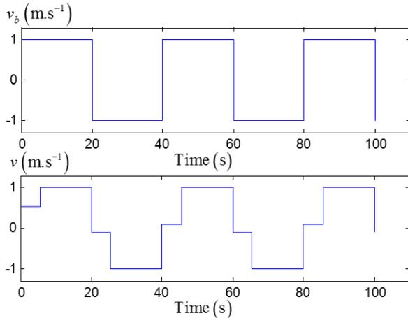
Fig. 6 (Top) Baseline velocity command. (Bottom) Shaped velocity command.
