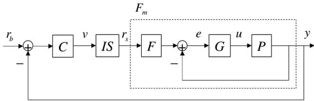
Fig. 1 Closed-loop signal shaping with inner-loop model matching.
