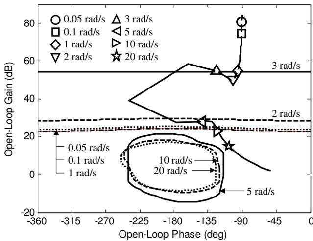
Fig. 4 Open-loop shaping: final shape.
