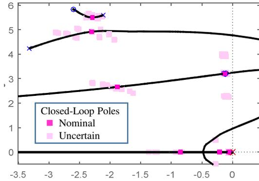
Fig. 9 Root locus plot without the inner-loop model matching.
