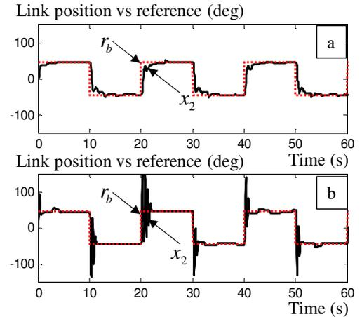
Fig. 16 Link position (in solid line) versus its reference (in dotted line). (a) Proposed CLSS with inner-loop model matching. (b) Traditional CLSS.
