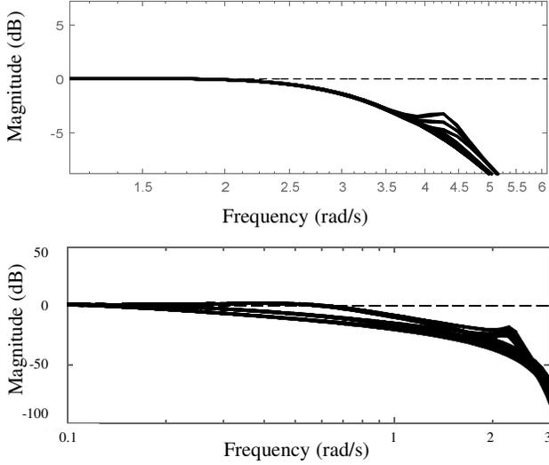
Fig. 8 Bode magnitude plots of the closed-loop systems. (Top) With the inner loop. (Bottom) Without the inner loop.
