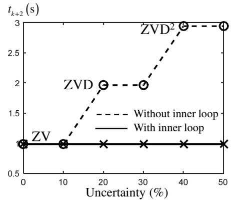
Fig. 7 Input shaper length as a function of uncertainty percentage: with and without inner loop.
