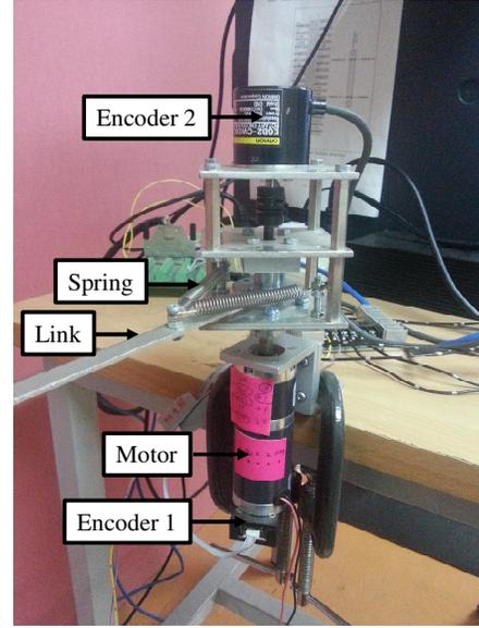
Fig. 12 Flexible-joint robot in the experiment.
