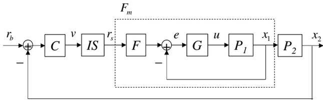
Fig. 14 Closed-loop signal shaping with inner-loop model matching.
