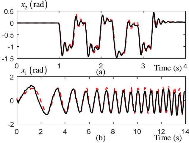
Fig. 13 System identification result. (a) Link position. (b) Motor shaft position.
