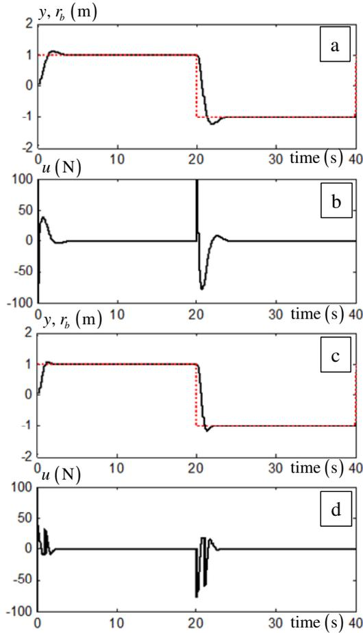
Fig. 11 Critically damped case: (a) flexible output and its reference and (b) control effort. Underdamped case: (c) flexible output and its reference and (d) control effort.
