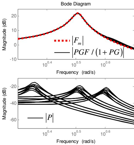
Fig. 5 Bode magnitude plots. (Top) With model matching. (Bottom) Without model matching.
