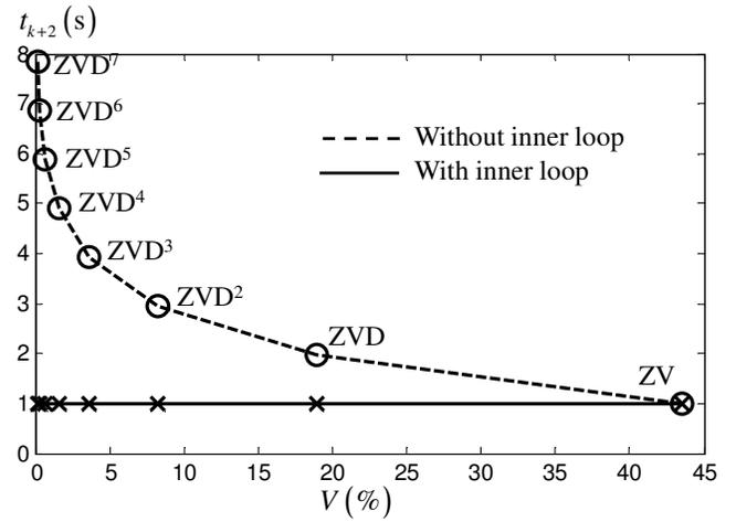
Fig. 6 Input shaper length as a function of percentage vibration: with and without inner loop.
