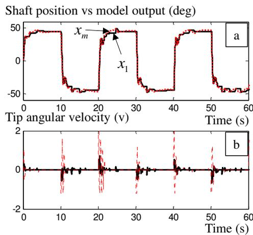
Fig. 18 (a) Motor shaft position (in solid line) versus reference model output (in dotted line) of the proposed technique. (b) Tip angular velocity of the proposed technique (in solid line) versus that of traditional CLSS (in dotted line).
