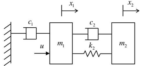
Fig. 2 Two-mass rigid-flexible plant.
