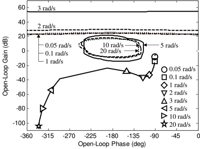
Fig. 3 Open-loop shaping: original shape.
