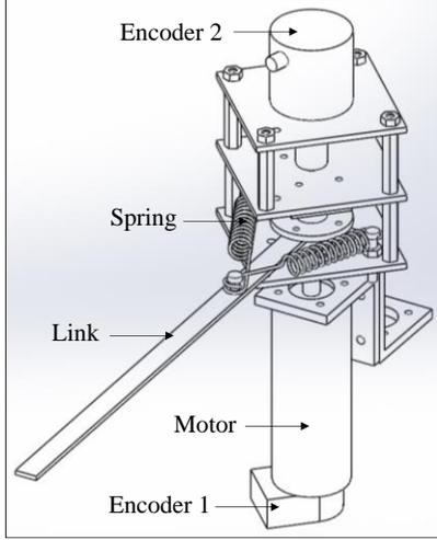
Fig. 6 Drawing of the flexible-joint robot in the experiment.
