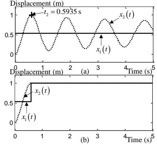
Fig. 5 Displacements  $x_1$  (in the solid line) and  $x_2$  (in the dotted line). (a) With the amplitude  $A_1$ . (b) With the amplitudes  $A_1$  and  $A_2$ .
