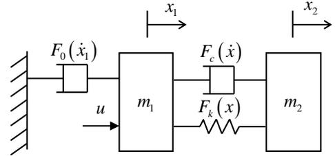
Fig. 1 Two-mass rigid-flexible plant with nonlinear spring and damper.
