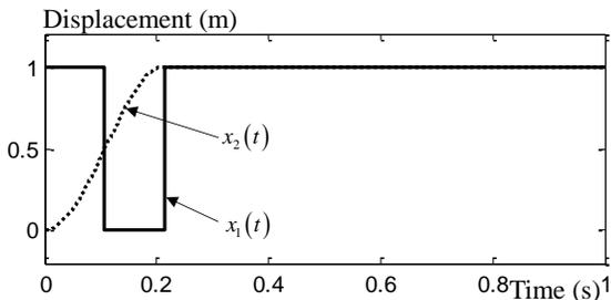
Fig. 12 Displacements  $x_1$  (in the solid line) and  $x_2$  (in the dotted line) using the negative input shaper.
