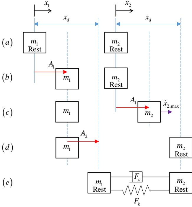
Fig. 3 Diagram of the two-mass system to design the input shaper.
