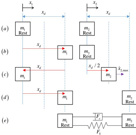
Fig. 11 Diagram of the two-mass system to design the negative input shaper.
