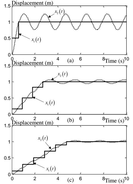
Fig. 10 Displacements  $x_1$  (in the solid line) and  $x_2$  (in the dotted line) when the mass  $m_2$  is 20% higher than its nominal value. (a) With  $n = 2$  impulses. (b) With  $n = 4$  impulses. (c) With  $n = 6$  impulses.
