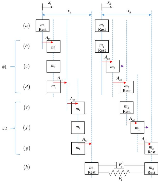
Fig. 9 Diagram of the two-mass system to design the robust input shaper.
