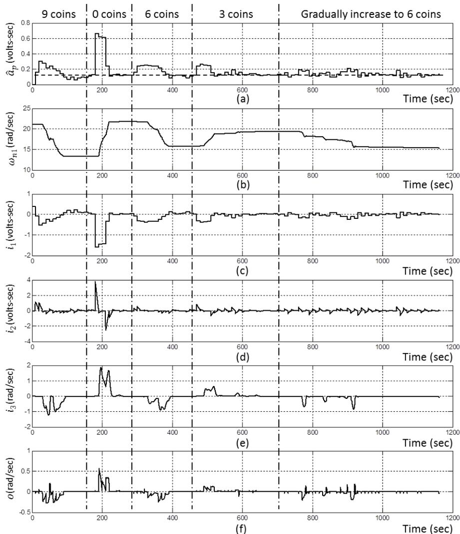
Fig. 10 Experimental results for adaptive input shaping. (a) Accumulated absolute acceleration  $\hat{a}_p$ . (b) First-mode natural frequency  $\omega_{n1}$ . (c) First input to the fuzzy system:  $\hat{a}_{pr} - \hat{a}_p$ . (d) Second input to the fuzzy system:  $\hat{a}_{pr}$ . (e) Third input to the fuzzy system:  $\omega_{n1}$ . (f) Output from the fuzzy system:  $\Delta\omega_{n1}$ .
