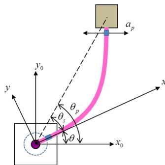
Fig. 2 Schematic diagram of the flexible-link robot.
