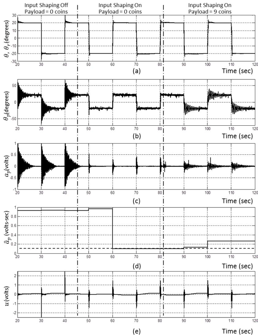
Fig. 7 Experimental results for un-adaptive input shaping. (a) Motor angle  $\theta$  and its reference  $\theta_r$ . (b) Payload angle  $\theta_p$ . (c) Payload acceleration  $a_p$ . (d) Accumulated absolute acceleration  $\hat{a}_p$ . (e) Control effort  $u$ .
