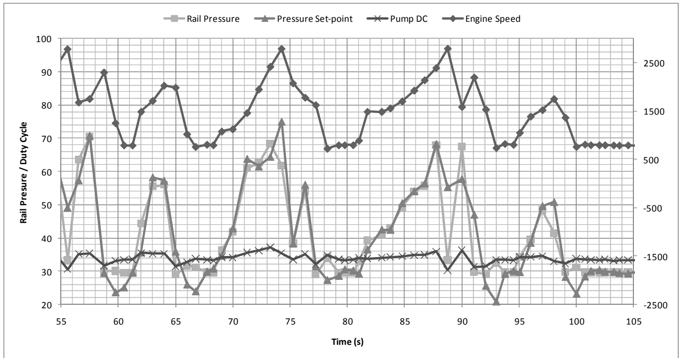
Figure 7: Road test on a pick-up truck using PID controller.
